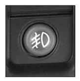
The fog lamp button is located on the left side of your instrument panel.
